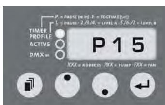
Fig. 5: Adjusting the performance of the fog generator
